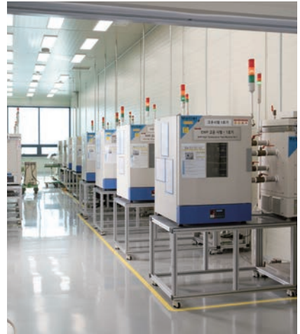
Electric water pump high-temperature durability tester
